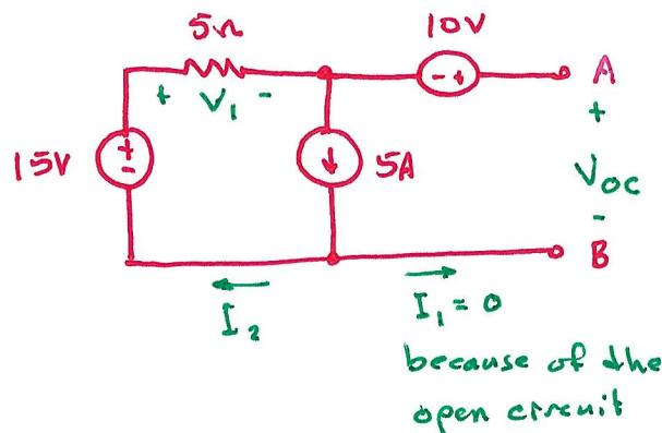
$$V_{oc} = 10V - V_1 + 15V = 0V$$
