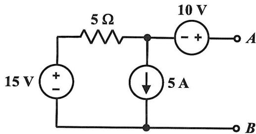
Determine the Thévenin equivalent circuit with respect to terminals *A* and *B*.
